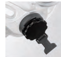
GP-7024C Air Valve for Mantis Full Face Mask After taking out the right or left cap on the mask, this breathing valve can be fitted on either side. Once the valve is fitted, without removing the mask, you can breathe outside air when you reach the surface or come ashore.
